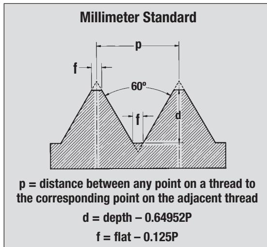
**p** = distance between any point on a thread to the corresponding point on the adjacent thread
